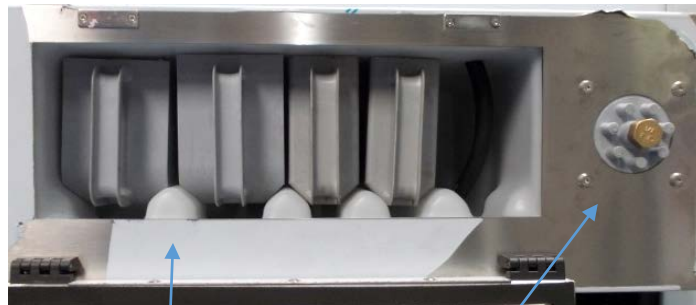
Detergent compartments and connection to dosing pumps (models 50 / 66)
